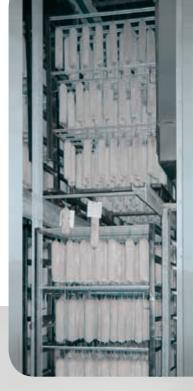
Optimally aligned salami maturing equipment for large production volumes and loading up to a height of 4.5 metres.
